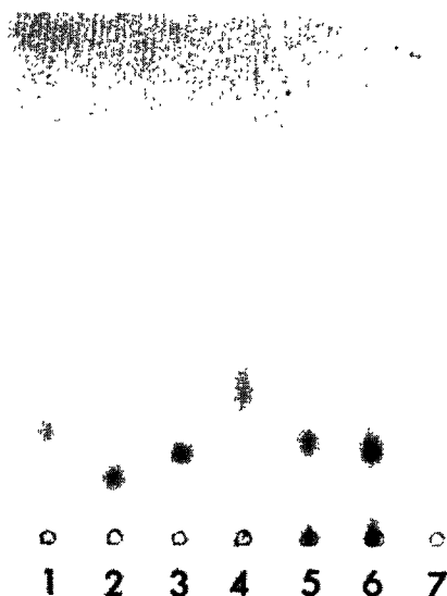
Fig.2. Chromatogram of sugars of the carbohydrate moiety of aspartyl-tRNA synthetase. Ascending thin-layer chromatography was carried out on a pre-coated silica gel plate using the solvent system ethyl acetate:propanol-1:propanol-2:water (8:5:1:1, by vol.). Numbers correspond to following spots: 1, mannose; 2, galactose; 3, glucose; 4, fucose; 5,6, aliquots of aspartyl-tRNA synthetase after exhaustive dialysis and hydrolysis at 100°C by 1 N HCl for 2 h and 2 N HCl for 4 h, respectively; 7, aliquot of the solution outside the dialysis bag containing the enzyme and treated by 2 N HCl for 4 h at 100°C.
